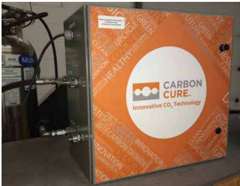
The CarbonCure technology precisely injects an optimized dose of liquefied CO 2 from a pressurized tank directly into a central mixer or truck at a dry batch plant.
