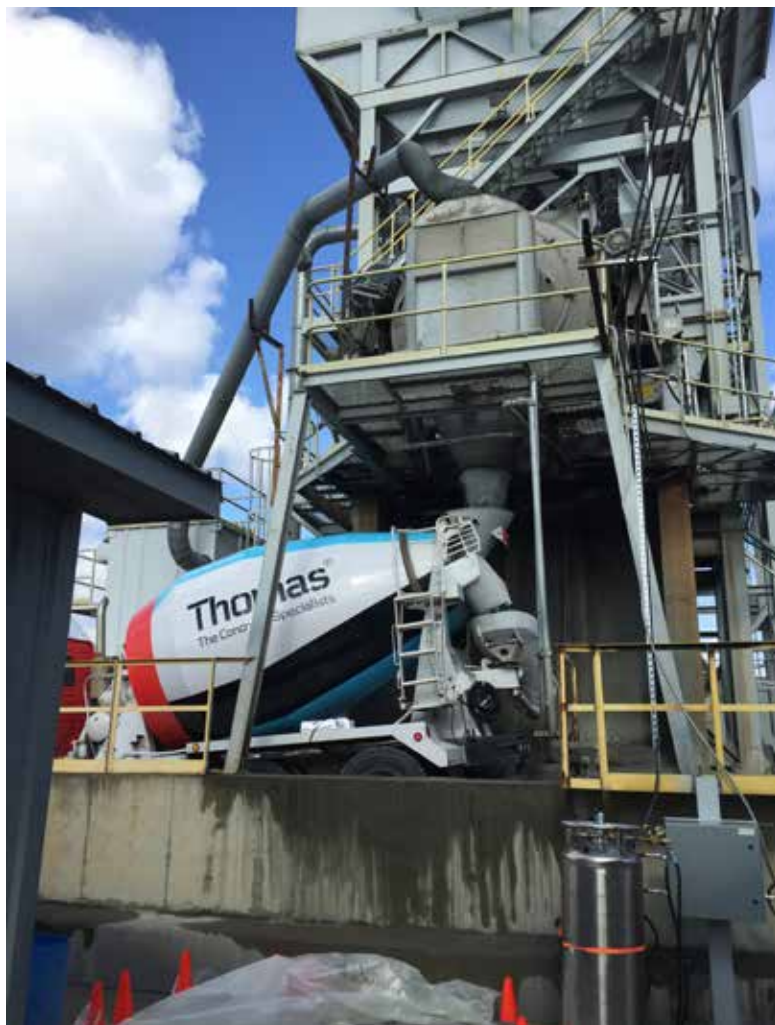
The CarbonCure technology precisely injects an optimized dose of liquefied CO 2 from a pressurized tank directly into a central mixer or truck at a dry batch plant.
